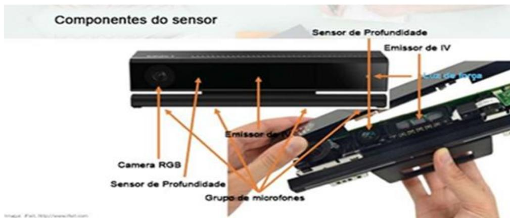
**Figura 2.5 – Componentes do sensor Kinect, adaptado de (KERKHOVE, 2014)**
